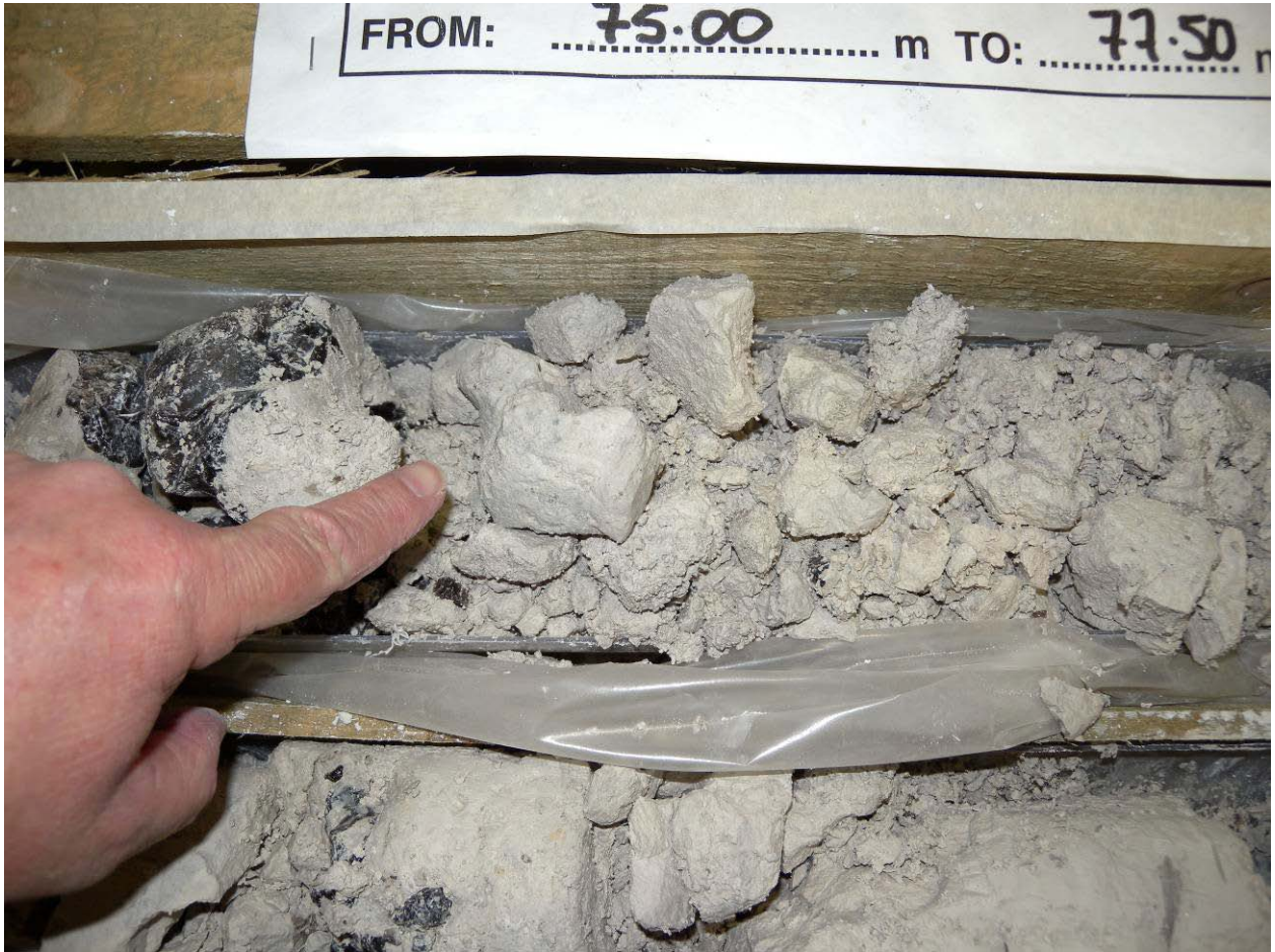
Interpreting drilling damaged core in terms of stratigraphy and engineering grade
