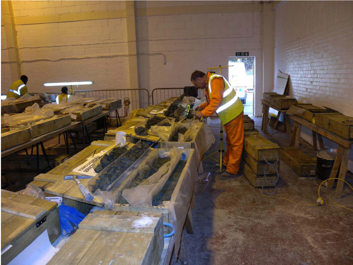
Logging the cores and check logging to ensure consistency
